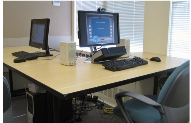
Figure 1: The high fidelity prototype, showing a welcome screen. The eye tracker is below the monitor.
