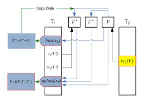
Figure 2: Ensuring isolation by replicating shared state and propagating appropriate copies using the resolution function *f*
