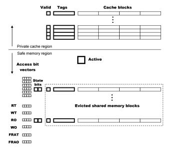
Figure 3: Basic structures of the proposed hardware for enforcing isolation (HEI)
