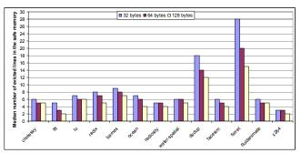
Figure 7: Median number of entries in the evicted cache of the safe memory required by HEI for different block sizes
