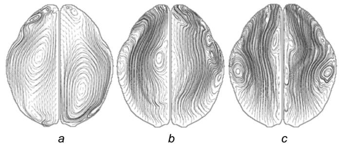
Fig. 2. The N-L CHI model—horizontal cross-section. Rotation about: center a, ear b; translation c.
