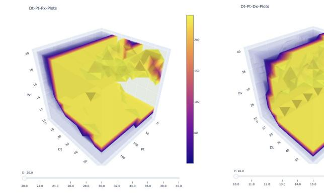
Surface-plot showing 4 control gains: Left keeping Dx fixed, Right Keeping Px fixed
