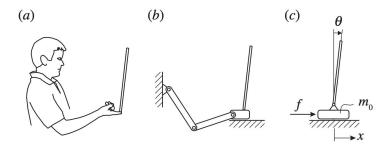
**Figure 1.** (*a*) Subject balancing stick on fingertip. (*b*) Slider crank model of the arm used to estimate the equivalent mass of the cart for the pendulum – cart model. (*c*) Pendulum – cart model for stick balancing with equivalent mass.
