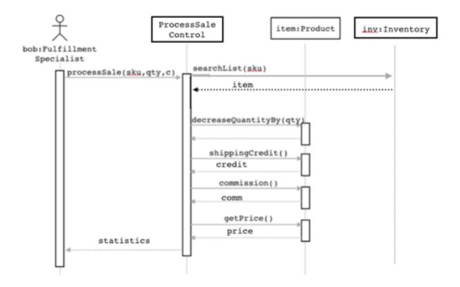
So the ProcessSaleControl communicates with the user and dispatches work to Inventory and Product. If I evaluate this with respect to the GRASP principles, it looks like ProcessSaleControl is doing a lot of work to compute the statistics (Low Coherence?). And the Product has all the information to compute the statistics, so maybe the Product should calculate the statistics by Information Expert:
