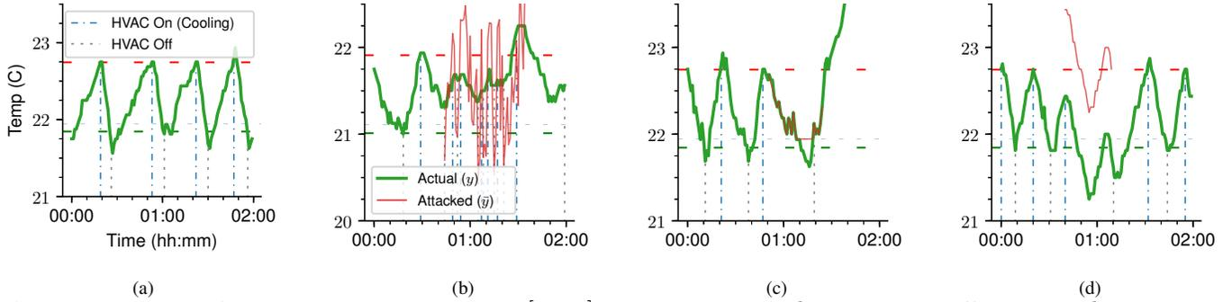
Fig. 9: Normal Operation (a); Fuzzy Attack: range =  $[-1, 1]$  (b); Clamp Attack:  $k = 21.94$  (c); Offset Attack:  $k = 1$  (d).
