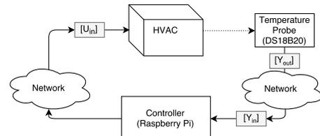
Fig. 8: HVAC Setup
