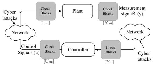
Fig. 1: A general block diagram for a CPS.
