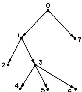
FIGURE 3. Pictorial representation of a tree rooted at 0. Each node has a unique predecessor except the root which has no predecessor.
