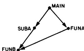
FIGURE 5. Illustration of the call graph for a FORTRAN program. The nodes have been labeled to identify the program unit represented.
