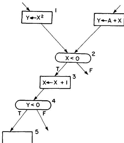
FIGURE 1. The path in this segment of a flow diagram represented by visiting the boxes in the sequence 1, 2, 3, 4, 5 is not executable. Note that  $Y \geq 0$  upon leaving box 1 and this condition is true upon entry to box 4, thus the exit labeled T could not be taken.
