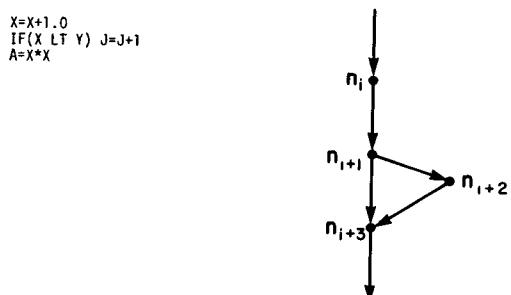
FIGURE 4. Graph representation of a segment of a FORTRAN program. Node  $n_i$  represents the statement  $X = X + 1.0$ , node  $n_{i+1}$  represents the first part of the IF statement  $IF(X.LT.Y)$ , node  $n_{i+2}$  represents the second part of the IF statement  $J = J + 1$ , and node  $n_{i+3}$  represents the statement  $A = X*X$ .
