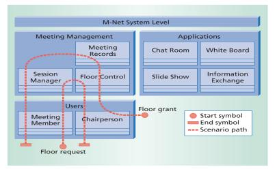
Figure 3. Initial grouping decisions and scenario mappings for an M-Net system-level module using a use-case map. The curved line represents a scenario's path as it weaves its way through the components with which it interacts.
