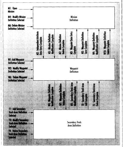
Figure 3. Object-communication diagram for the Mission Generation System. Each object is shown as a rectangle; connecting arcs are labeled with communicating events.
