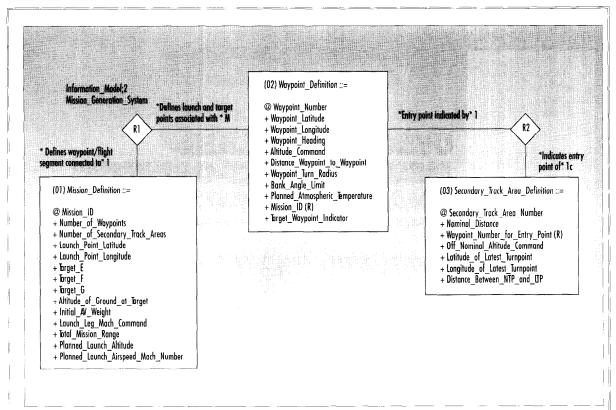
Figure 1. The information model for the Mission Generation System. The information model has both textual and graphical representations. A textual representation consists of a set of textual definitions (semantics) for each object, attribute, and relationship describing the basis of abstraction. The graphical representation provides a global view of the entire MGS.
