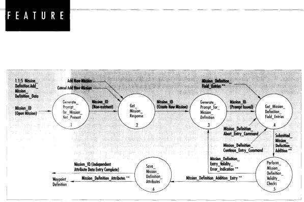
Figure 4. Dataflow diagram for the the mission object state "Enter Mission Definition Data State." Each circle in the diagram represents an action process of a given state. The dataflow diagrams contain processes (like Get\_Mission\_Response), data stores, dataflows (like Mission\_ID, which creates a new mission), and a number of sources and sinks.
