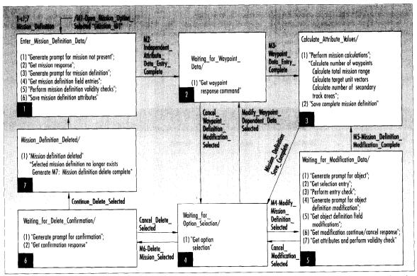
Figure 2. The life cycle of the mission object shown as a state-transition diagram, in which each state and its I/O are maintained separately. The rectangular boxes show different states. Arrows indicate transitions during an event.
