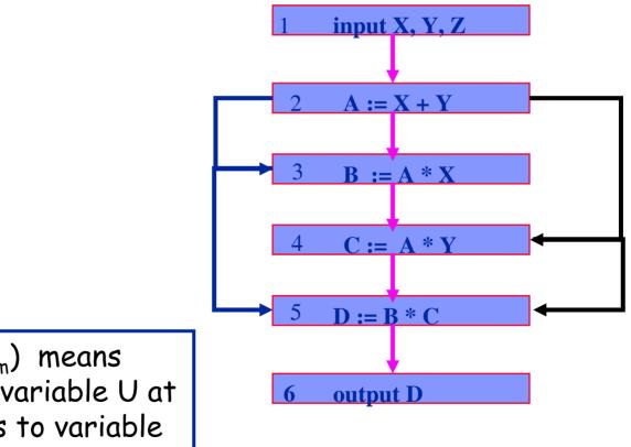
Notation:  $(U_n, V_m)$  means faulty value for variable U at node n transfers to variable V at node m
