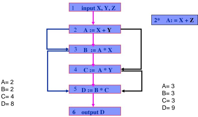
test case: x=1, y= 1, z=2 satisfies the conditions  $x \neq 0 \land y \neq 0 \land y \neq z$ and causes the fault to be revealed
