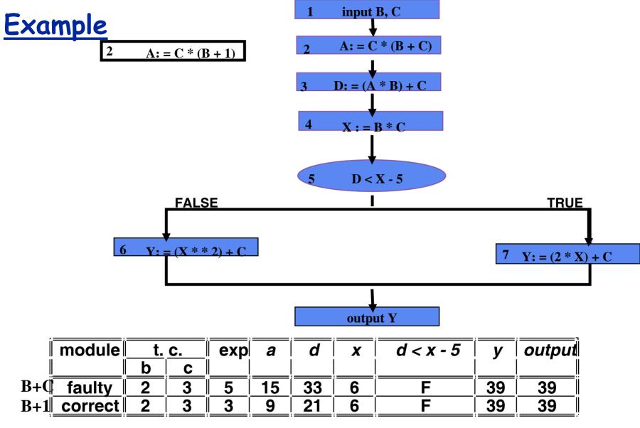
ORIGINATION, COMP. TRANSFER (NODE 2) DATA DEPENDENCE TRANSFER (NODE 3) NO DATA DEPENDENCE TRANSFER AT NODE 5
