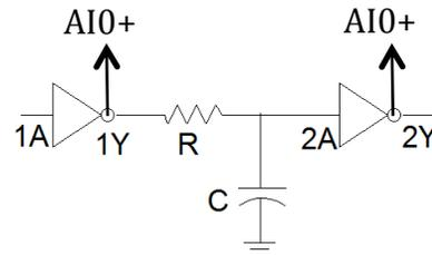
To understand the propagation delay, we put a resistor of  $1\text{k}\Omega$  and a capacitor of  $1\mu\text{F}$  between 1Y and 2A, so that the delay is amplified and observable by NI Elvis.
