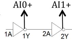
Connect pin 1Y to channel AI0+ and pin 2Y to AI1+ on the upper left side of the board. Finally connect channel AI0- and AI1- to the Ground channel.
