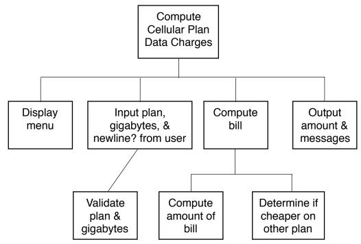
The Top Down Design chart does not specify control flow. It does not specify looping or branching. Sometimes the code to carry out each task ends up being interleaved in the final program. In this program the input from the user and output to the file are interleaved. Also, the tasks are performed once for each rat, and the design doesn't specify what kind of loop to use (count-controlled, sentinel-controlled, etc.).
