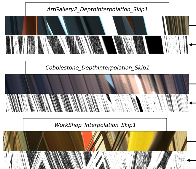
Figure 4.1.5: Example EPIs and their corresponding Canny edge maps for an LFI from the MPI dataset [7].
